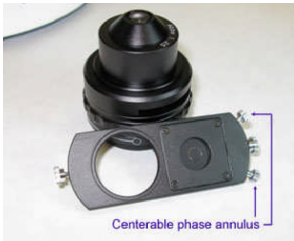
Abbe Condenser NA 1.25 with iris, centerable 20x & 40x positive phase annulus
